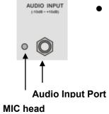
Audio signal can be taken from mixer controller, line level output of other audio equipments, or MIC input. Controller automatically extracts low-frequency component from music as music trigger synchronous signal for Multi-Step-Program program.
