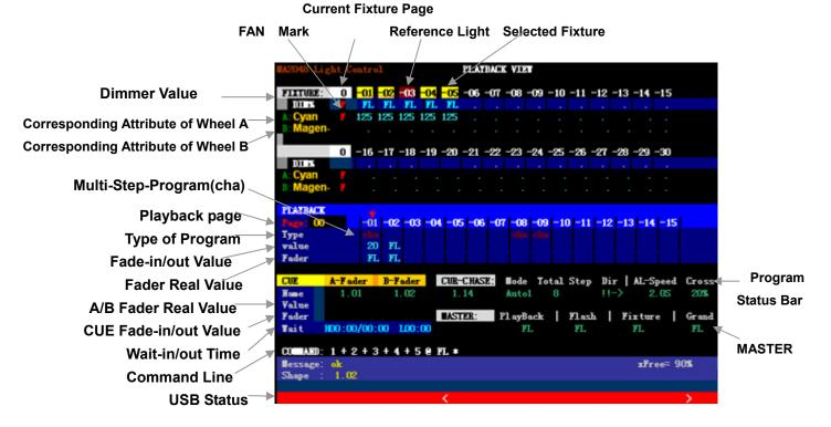
EXP8000 Intelligent Fixture Controller is displayed on VGA1 monitor and also on VGA2 monitor, through which, output value of channels of DMX singal from controller can be
