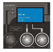
2) A/B Wheel is primarily used to set various attribute values of fixture.
