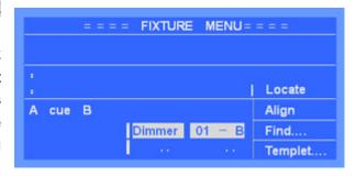
(Locate has an important function that various attributes of selected fixtures are assigned a value, which is of great significance for enforcement of the Rule of LTP (LATEST TAKES PRECEDENCE).
