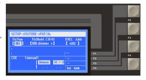
shown on the above of major display screen (shown as the right). To return last layer of menu, press **BACK** key, to return Scene menu, press the current Main Menu Key once again till the flickering indicator light is off, which means returning to live show menu.
