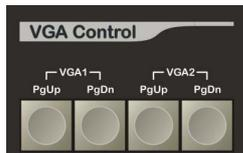
Through keys on VGA Control, to view page by page on externally connected VGA monitor can be realized. Under different menus, VGA1 outputs differently. Screen can be turned up and down through the corresponding PgUp/PgDn key. VGA2 displays the numerical value outputted by DMX and also screen can be turned up and down through the corresponding PgUp/PgDn key.
