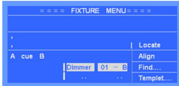
(Locate has an important function that various attributes of selected fixtures are assigned a value, which is of great significance for enforcement of the Rule of LTP (LATEST TAKES PRECEDENCE).
