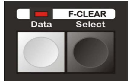
Clear key can only clear all values of Manual-run while unable to clear the designated value of Manual-run, when the designated fixture is to be cleared by users, the commands such as follows can be used:
