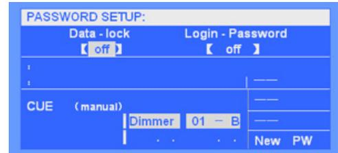
**Steps:** press **New PW** (LCD displays **Enter New Password**). Enter new password and then press **ENTER** key (only number can be for password and also be as power-on password).
